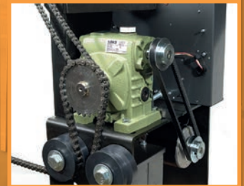
Full Size Gearbox heavy-duty 30:1 ratio gearbox
